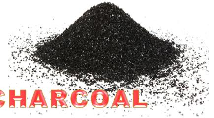
Activated charcoal is produced from the controlled burning of wood, which is then subjected to the action of an oxidizing gas such as steam or air. This process enhances the adsorptive power of charcoal by developing an extensive internal network of fine pores in the material.
